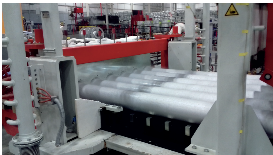
Horizontal continuous casting machine
