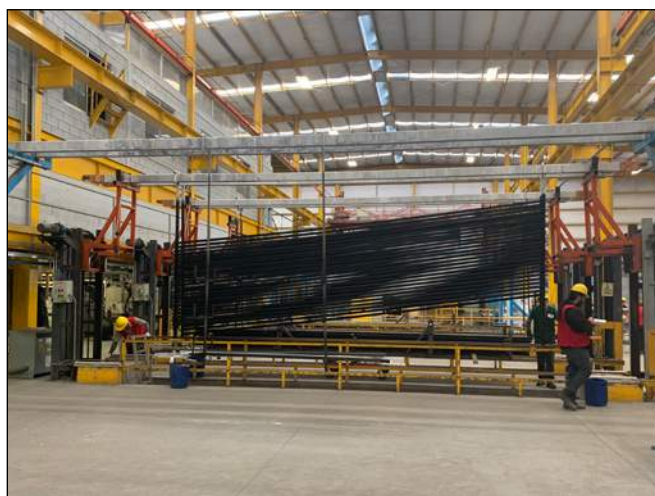
Figure 3. The anodizing line primarily processes profiles for the solar market.
