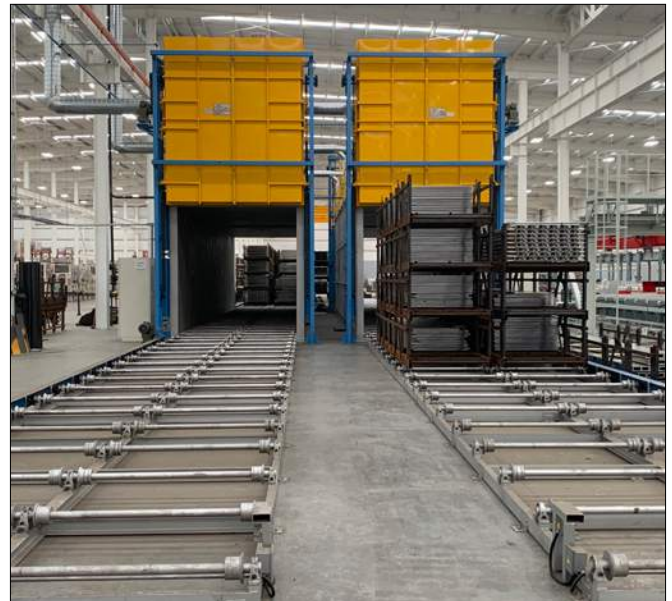
Figure 8. Aging ovens heat treat profiles to meet customer specifications.
