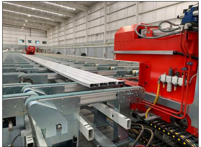
Figure 6. The 150 ton, fully automated stretcher.
