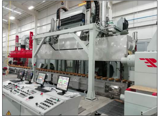
Figure 5. A multi-zone quench provides both air and water cooling.
