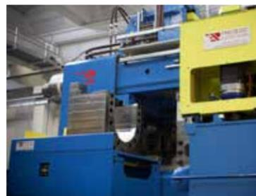
This solution was decided in order to keep the existing smaller press, that is able to extrude smaller profiles, on the same footprint optimizing the space available. The state of the art cooling and quenching system at the press exit, can work with intensive air or intensive water according to the required metallurgical and mechanical
