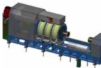
In the ZPE all components that are subject to the magnetic field, are made of non-magnetic material, so as not to compromise the operation.
