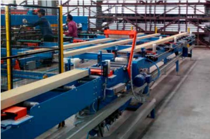
The packing line consists in an innovative system of loading and unloading of the baskets that, thanks to its special 2 levels layout, allows to optimize the spaces and to reduce the waiting time of the operators. The very packaging part is composed by a profile wrapping line for high levels of production and by a semi-automatic strapping line, particularly effective for its reduced dimensions and for its functional simplicity.
