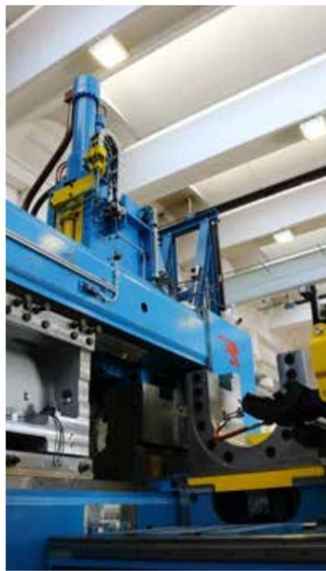
machine, as the main motor unit, the puller jaw rotation, jaw height adjust and IN/OUT of the jaws are foreseen by means of AC drives with frequency converter installed on board of the carriage.
