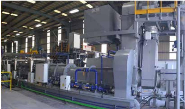
front loading press and a COIM log furnace with hot saw.
