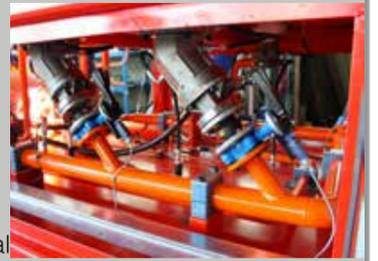
PE. E.E.S. system allows the press to generate only the exact force and speed needed for the particular extrusion operation as and when it is really required. Pumps that are not needed during the extrusion phase are completely at rest.
